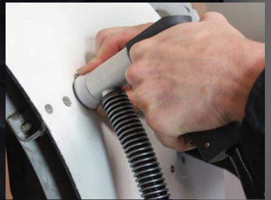
Targeted blast with debris recovery
